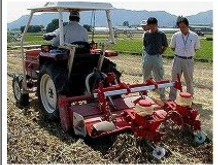
The Shallow Tilling and Ridging Seeder Method – a new farming system for soybean cultivation
